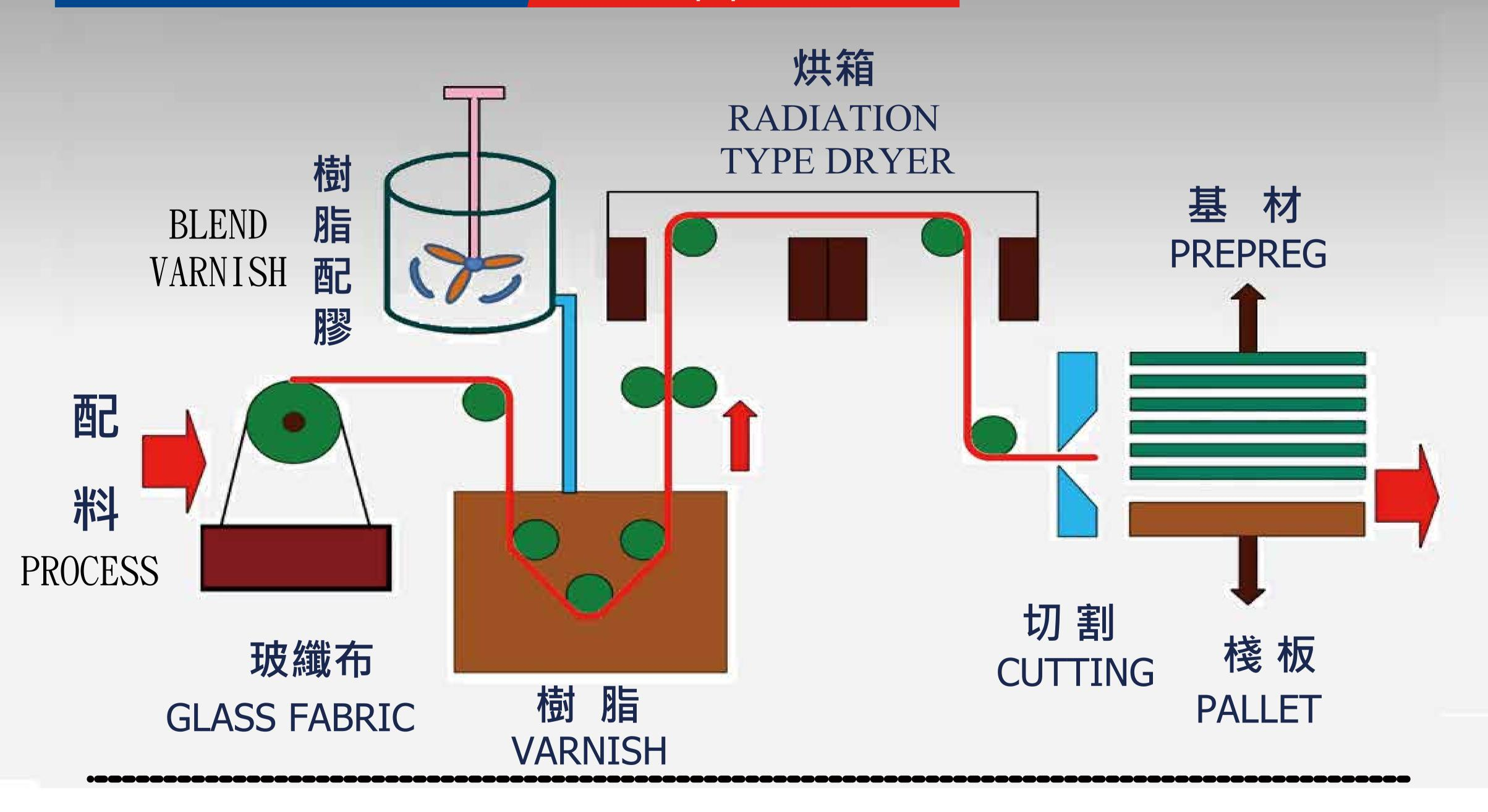
The glass fiber cloth is impregnated with resin, and heat energy is used to volatilize the solvent to carry out a bridging reaction and become a semi-hardened substrate.
